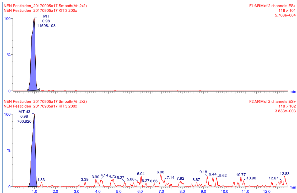
Figure 23: CMIT and CMIT-d3 in an undiluted sealant extract
